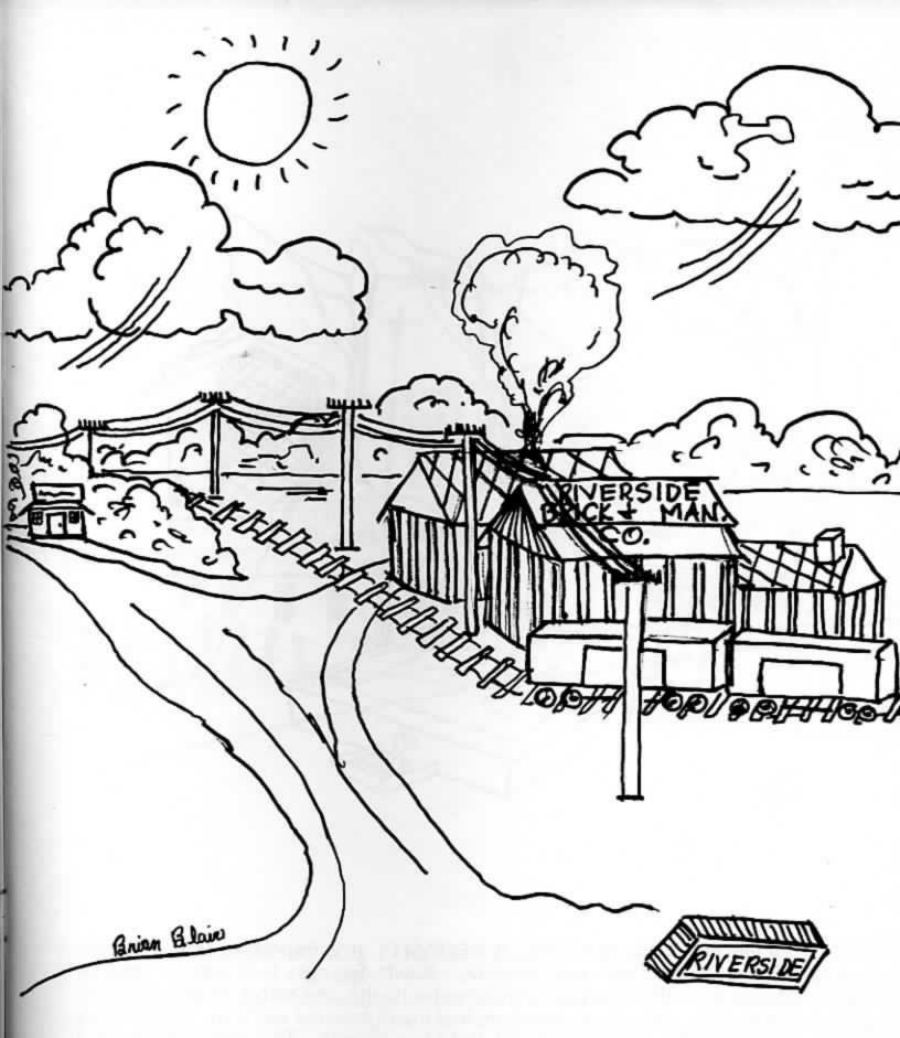
BRICKS WERE DRIED BY WOOD FIRES IN UPDRAFT KILNS AT RIVERSIDE. The clay used to make the bricks was found near by. After fire destroyed 26 business houses in 1893, downtown stores were rebuilt with brick and stone. Bricks were used to pave early streets. **LOOK FOR** old bricks marked "RIVERSIDE".
